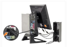
7 Connect the USB, keyboard and mouse cables to the computer as shown.
