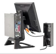
**5** Connect the power cable to the monitor as shown.
