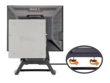
3 Tighten the screws underneath the stand.
