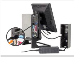
6 Connect the power adapter firmly to the computer as shown.
